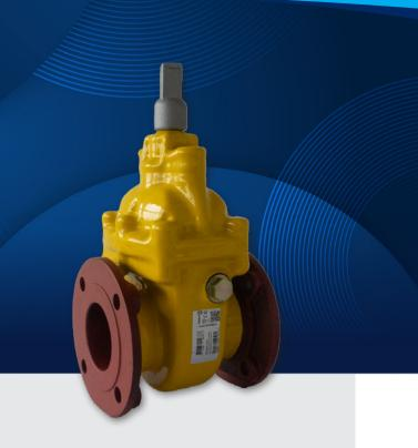
The Series 555/401 softseal valve is a double-faced, resilient seat, internal screw, clear bore wedge gate valve. It is designed primarily for the isolation of natural gas and manufactured gas underground. Manufactured with the new Donkin PUR corrosion protection system, enabling burial without need for wrapping of the valve body. To ensure full long term protection, flanges and bolts should be wrapped in line with industry guidelines. Manufactured and approved to specification GIS/V7-1.
